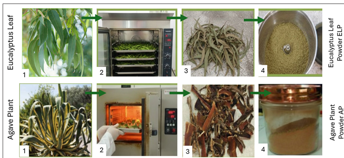
Figure 2. Preparation of eucalyptus leaf powder and agave powder: (1) plant harvesting (2) oven drying (3) dried plants (4) grinding
