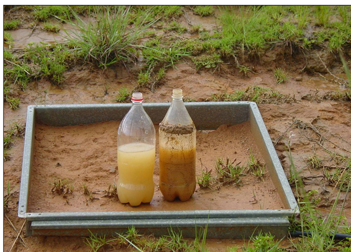
Figure 6. Runoff water quantity and quality on slopes are assessed using runoff plots
