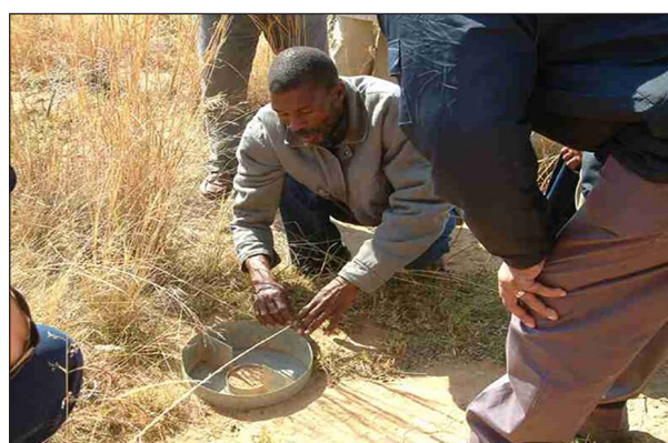
Figure 3. A Morgan splash cup used to quantitatively measure up- and downslope erosion
