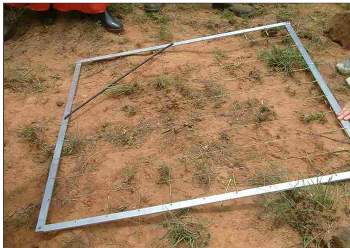
Figure 5. Plant basal cover is assessed using a one square metre quadrat subdivided into 100 squares
