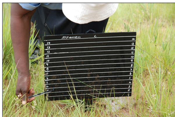
Figure 2. Splash board showing the extent of soil detachment as a result of rain splash
