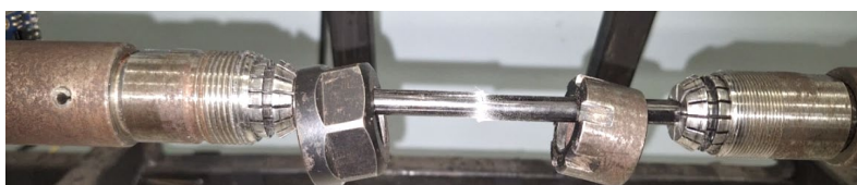
Figure 16: Specimen failure in collet assembly
