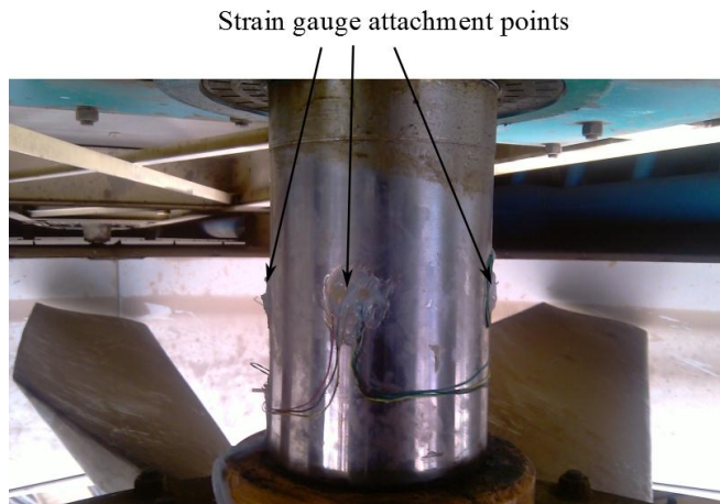
Figure 6 Strain gauges attached to fan shaft
