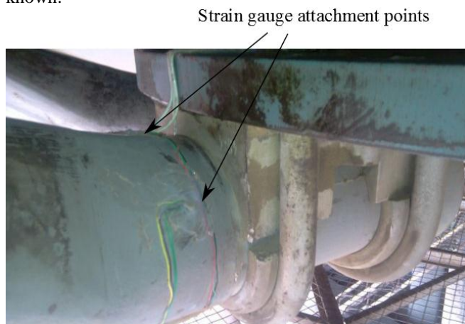
Figure 5 Strain gauges attached to fan blade
