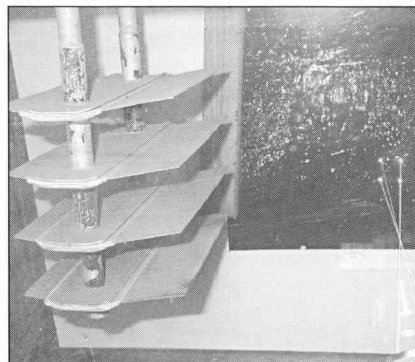
Fig.4: Sideview of the oscillator and look at the four laser beams of the 2D LDA-optics
