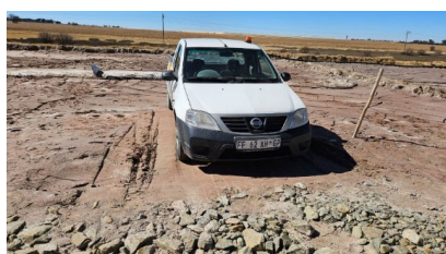
Figure 12—The ATA® buttress could support a vehicle being driven onto and off the buttress 13 days after deposition
