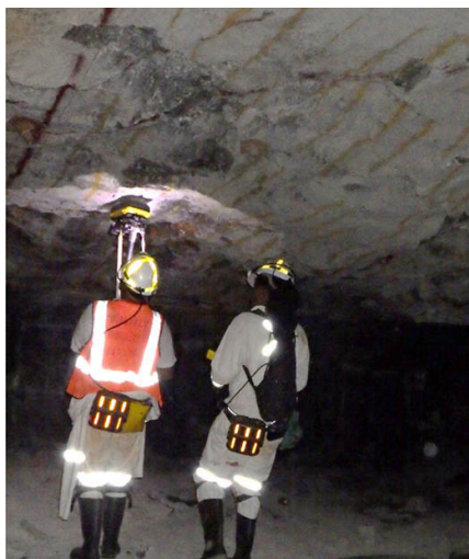
Figure 4—Acquisition of GPR data along the marked hanging wall grid intervals between each successive survey line. The GPR data was acquired by using a RockNoggin 1 GHz GPR system, manufactured by Sensors & Software (Sensors & Software, 2023). During data collection along the hanging wall area, a Smart Handle attachment was employed to effectively deploy the GPR antenna along the hanging wall surface, as depicted in Figure 4, ensuring precise data acquisition.
