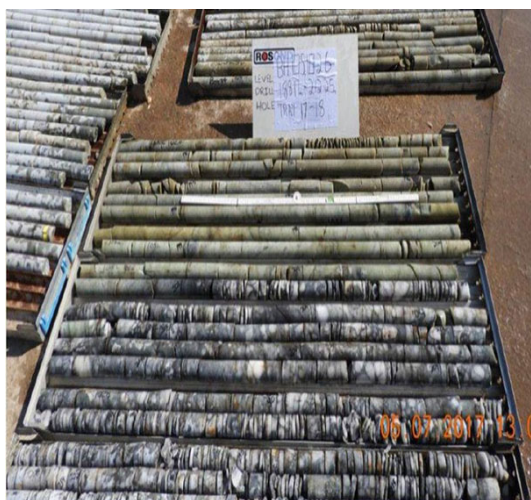
Figure 7—Rock fracturing ahead of a mining face, as observed from mine drill core after destress blasting (Sengani, Zvarivadza, 2018a)
