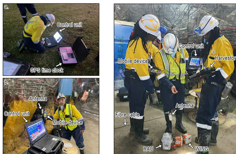
Figure 4— (a) The GPS time system is synchronised with satellites for underground tunnel use, providing signals to (b) Mobile devices at 3000 m below the surface, and (c) Fed to nodal systems
