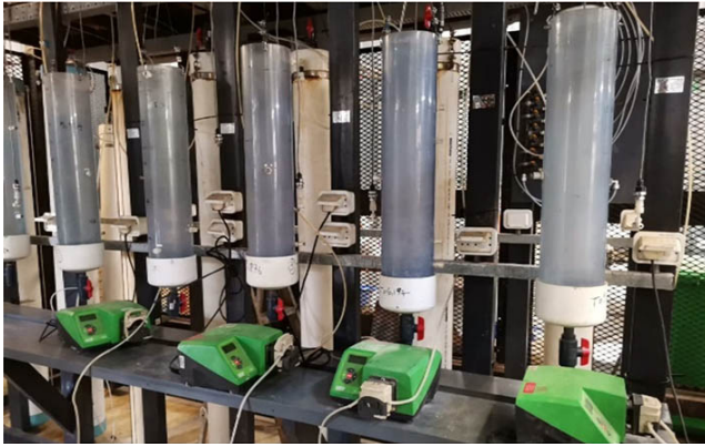
Figure 1—Hydrodynamic column test apparatus
