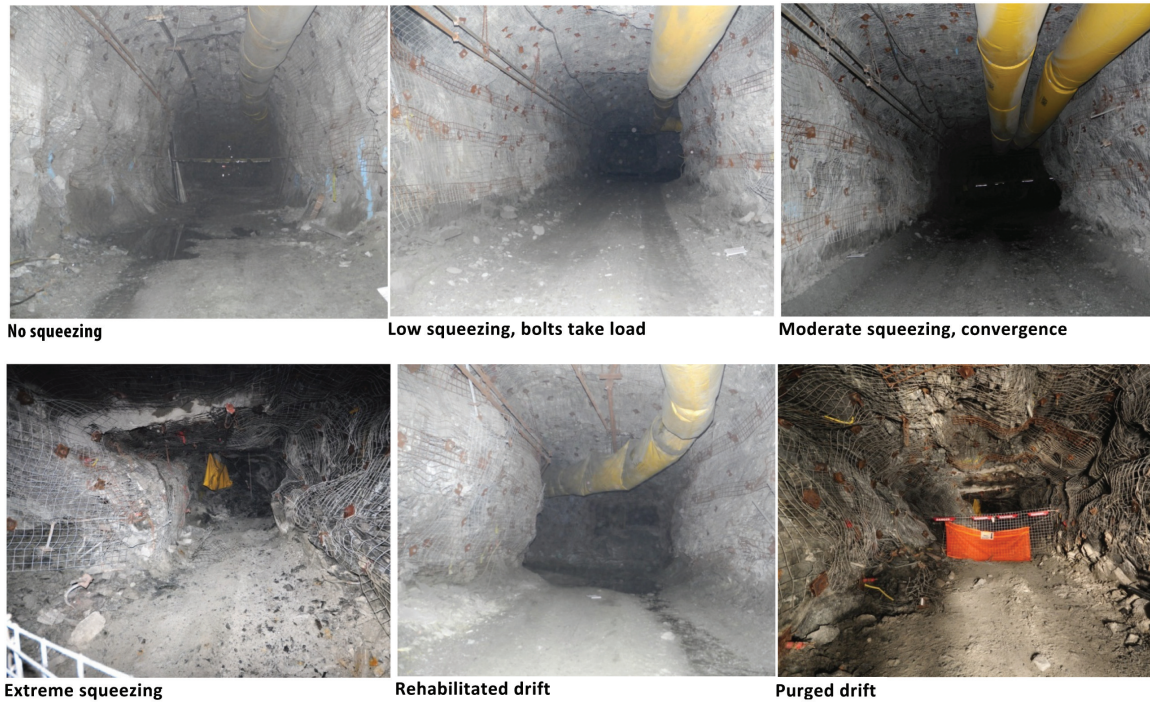
Figure 5 – Examples of drifts subjected to squeezing at the LaRonde and Lapa mines (Hadjigeorgiou et al. , 2013)
