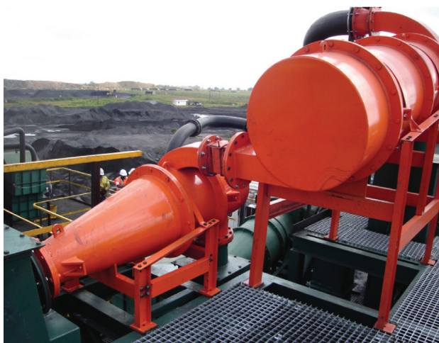
Figure 2 – 3-product cyclone at Umlalazi Mine
