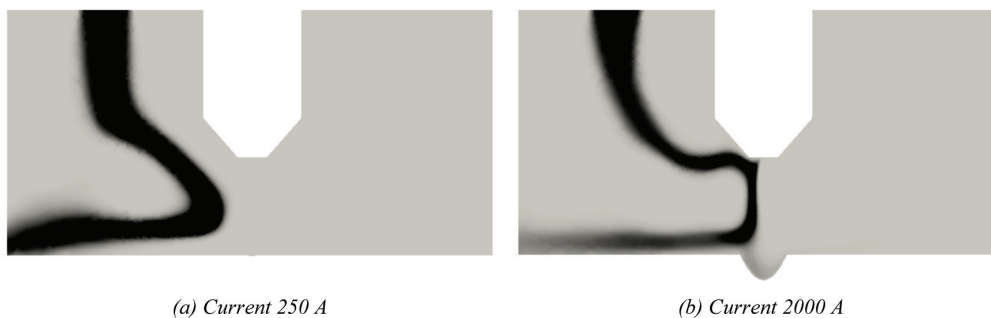
Figure 8 – Steady-state dust concentration fields at various currents. Scale 0 (grey) to 0.5 (black) kg/kg
