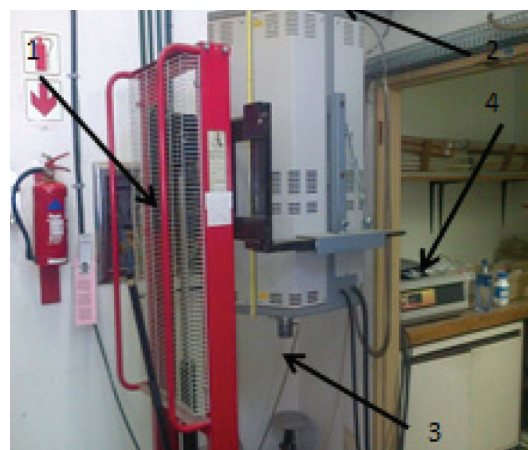
Figure 1 – A Carbolite STF 1800 tube furnace with controller after being modified with a fork-lifter. (1) Fork-lift, (2) argon gas inlet, (3) gas outlet with extraction fan, (4) temperature controller
