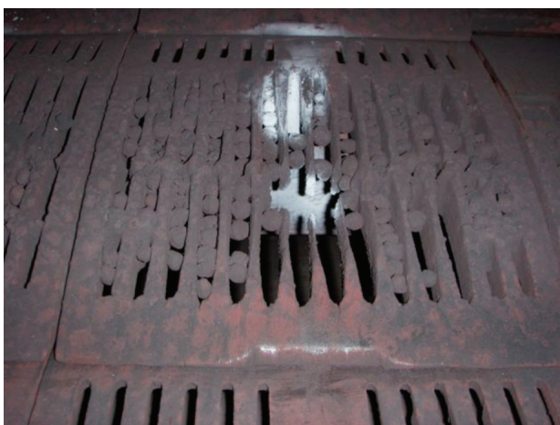
Figure 6b—Grate plate, worn-out
