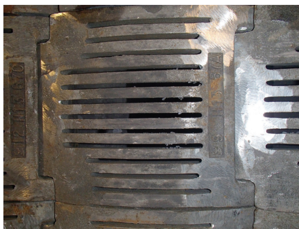
Figure 6a—Grate plate, as produced
