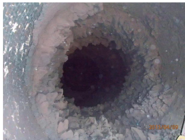
Figure 5—Accreted chunks in a rotary kiln (Svappavaara, Sweden) during a maintenance stop in 2013
