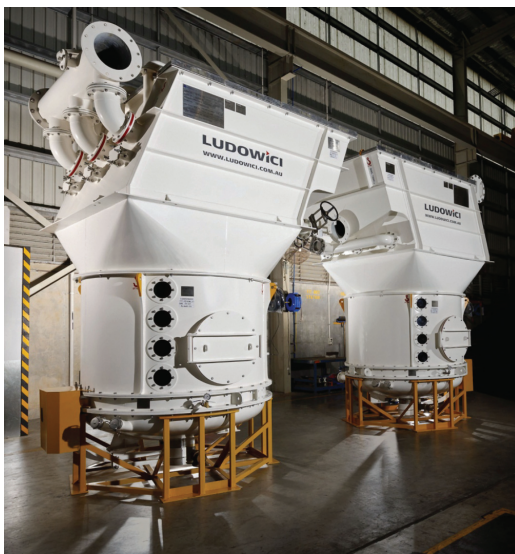
Figure 5—RC™2000 REFLUX™ classifiers factory test assembly prior to delivery
