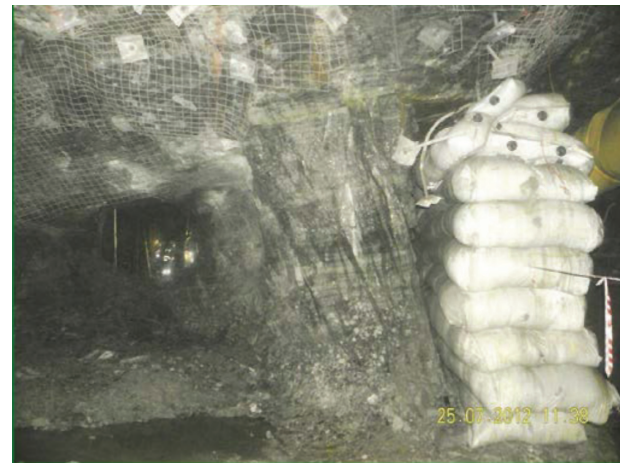
Figure 26—Narrow edge of a crush pillar showing the fracturing in the pillar. A PoweRite backfill bag is shown on the right of the pillar
