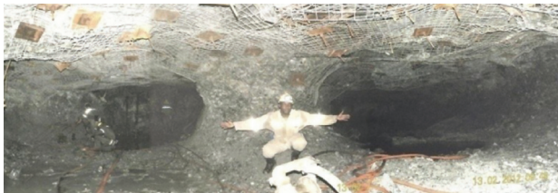
Figure 25—Panoramic view of a crush pillar layout
