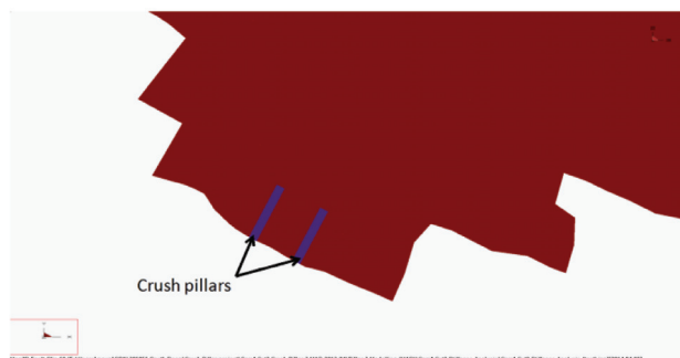
Figure 16—Plan view of the stope (red) and modelled 'crush' pillars
