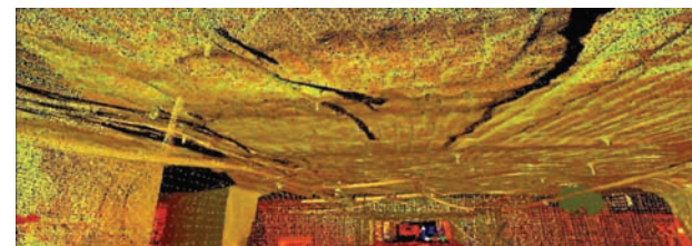
Figure 12—One scan reveals a vast amount of detail – support, geological features, vent seals, etc.
