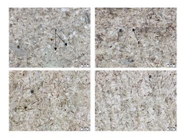
Figure 6—Microstructure of BN1 at a cooling rate of (a) 4°C per second showing ferrite (F), bainite (B), and martensite; (b) 6°C per second showing ferrite (F), bainite (B), and martensite; (c) 7°C per second showing ferrite (F), bainite (B), and martensite; and (d) 15°C per second showing ferrite (F), bainite (B), and martensite (M)
