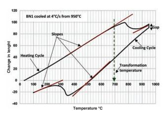
Figure 4—A typical change in length vs. temperature curve for Alloy 1 at a cooling rate of 4°C per second showing the relevant slopes. The dashed vertical line shows where the transformation temperature for  $A_{\rm c1}$  would be taken, i.e.  $700^{\circ}\text{C}$
