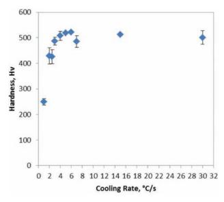
Figure 10-Hardness (Hv) vs. cooling rate (°C per second) graph for BN1
