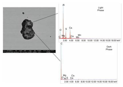
Figure 8—(a) SEM micrograph showing the dark and light phases of an inclusion found in BN1 cooled at 7°C per second and (b) EDX analysis of the
