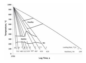
Figure 9-CCT diagram for BN1 showing the martensite, bainite, and pearlite regions
