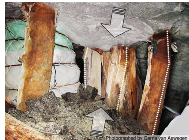
Figure 13—Buckling of timber elongates consistent with the implied direction of dynamic stope closure. Closure of up to 130 mm was measured while the elastic convergence was ~20 mm as indicated by numerical modelling
