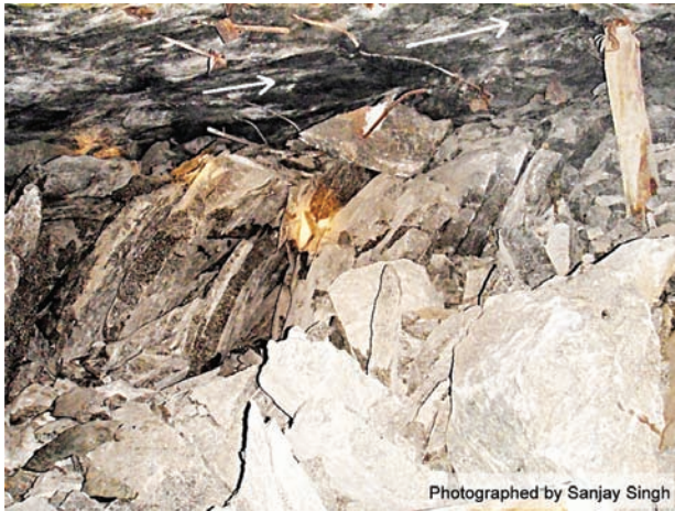
Figure 14—Ejection of the pillar edge (Case 4) along a plane of weakness in the stope hangingwall. The ‘naked tendons’ are pulled in the direction of ejection, pointing in the same direction as slip striations (white arrows) along the plane of weakness
