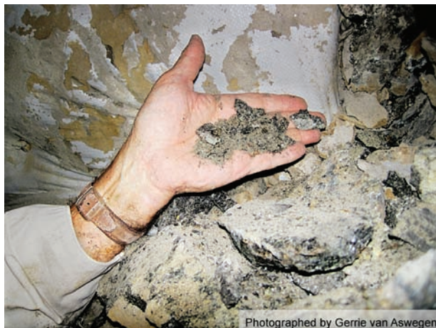
Figure 11—Comminuted Merensky Reef illustrating dynamic failure of the pillar in Case 3
