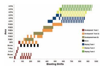
Figure 3—Mining rate for down-dip mining
