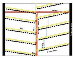
Figure 2—Layouts for down-dip and breast mining
