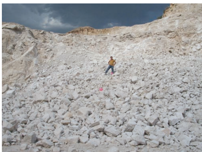
Figure 6—Rock pile of blast round with drill cuttings stemming at Bozanonu limestone quarry
