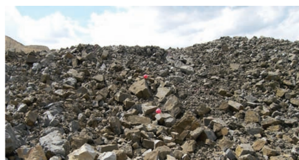
Figure 4—Rock pile from blast round with drill cuttings stemming at Goltas clay quarry
