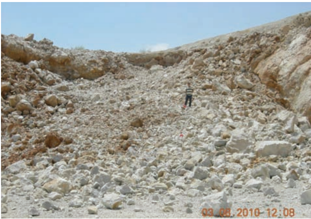
Figure 10—Rock pile of blast round with drill cuttings stemming at Bastas limestone quarry
