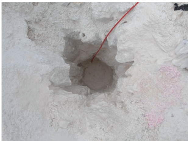
Figure 3—Cracked hole collar and hardened plaster
