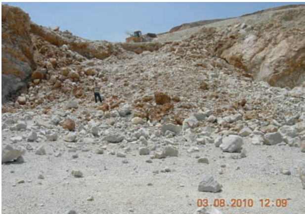
Figure 11—Rock pile of blast round with plaster stemming at Bastas limestone quarry
