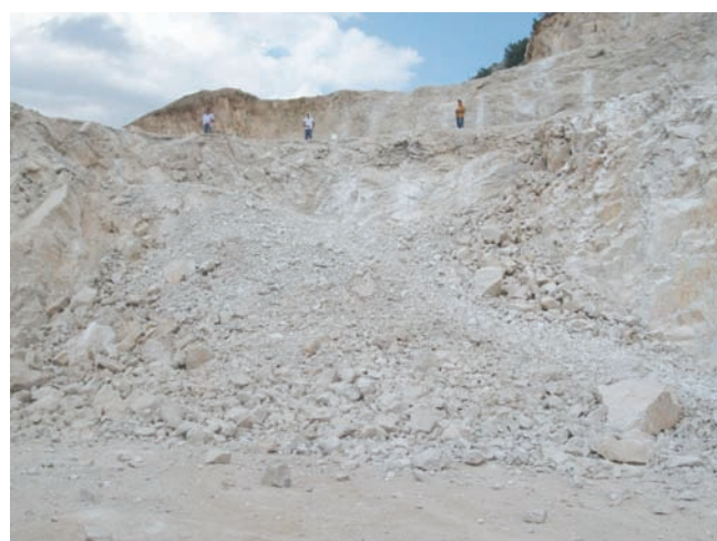
Figure 7—Rock pile of blast round with plaster stemming at Bozanonu limestone quarry
