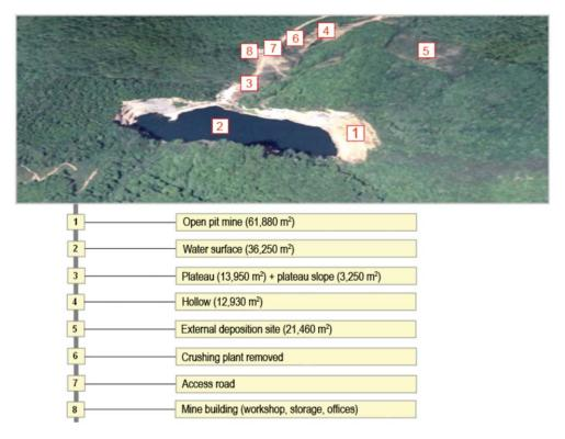
Figure 2—Orthophoto snapshot of the 'Srebro' open pit mine area
