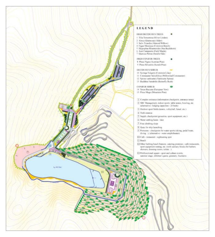
Figure 5-Plan of spatial arrangement and vegetation at the open pit mine and the mine plateau
