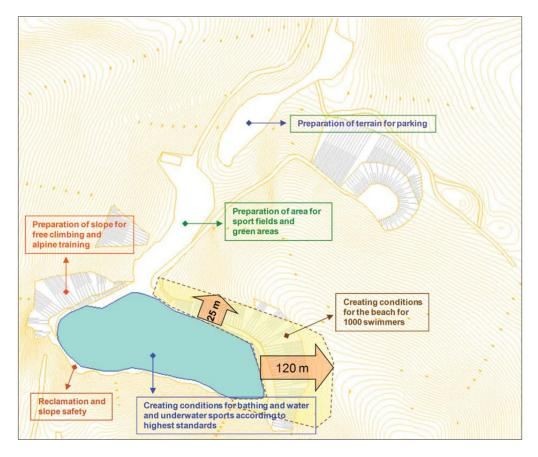
Figure 3—Plan of moving open pit mine boundaries and purpose of space
