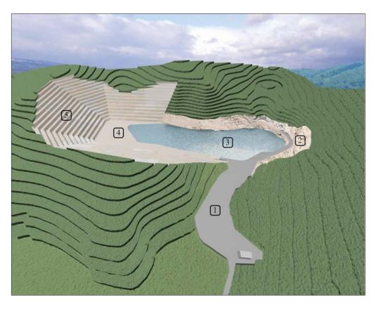
Figure 4—Outline of the contour and surroundings of the open pit mine after completion of the technical land reclamation (3D MODEL), (1)—mining plateau; (2) free climbing area; (3) lake; (4) beach; (5) amphitheater
