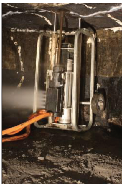
Figure 14—Autorock drilling 90° support holes in a platinum mine stope in the Rustenburg area
