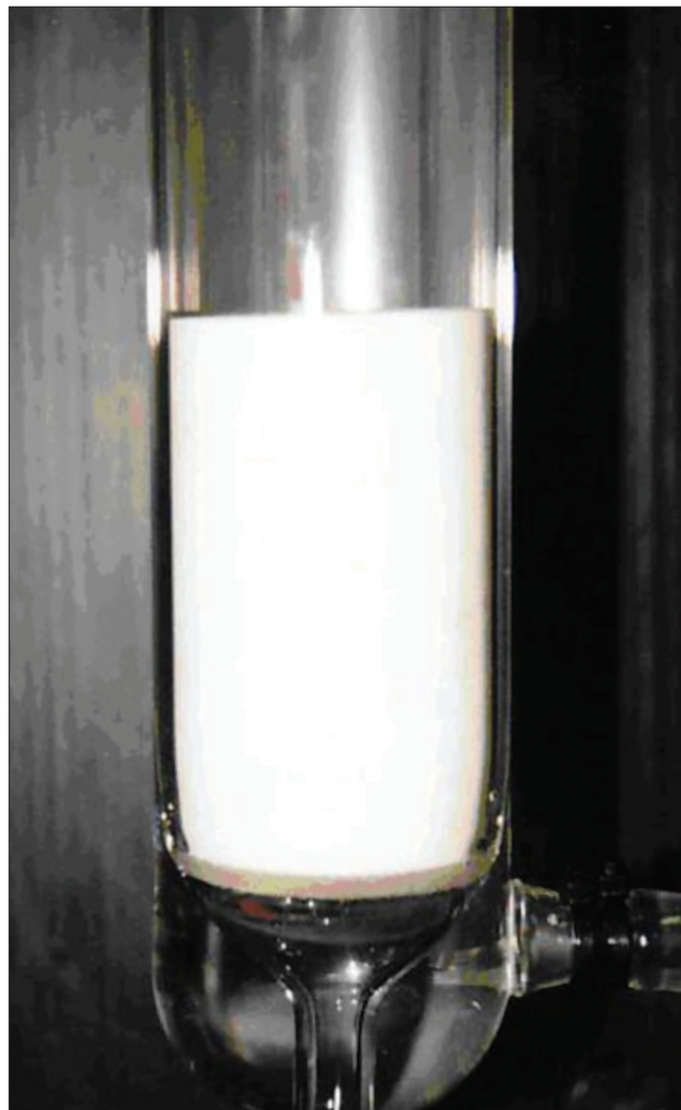
Figure 1—Jacked column packed with activated alumina used for the adsorption-desorption cycle
