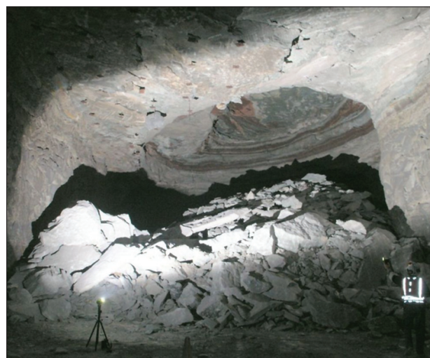
Figure 4—Large-oval shaped fall that has propagated upwards into weaker overlying strata in a limestone mine
