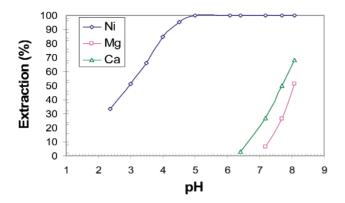
Figure 5—Extraction pH isotherms of Ni, Mg and Ca by a mixture of 0.5 M V10 and 0.5 M LIX®84-IC in xylene at 40°C with O:A = 1:1
