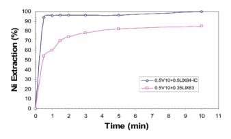
Figure 12—Nickel loading kinetics for V10-LIX@63 at O:A ratio 1:1 and V10- LIX@84-IC systems at  $40^{\circ}$ C with O:A = 1:2 at pH 5.00
