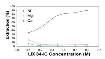
Figure 10 – Effect of LIX $^{\odot}$ 84-IC concentration on Ni, Mg and Ca extraction at pH 4 and T =  $40^{\circ}$ C
