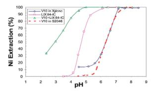
Figure 7—pH dependence of 0.5 M V10 in xylene, 0.5 M LIX®84-IC in xylene, 0.5 M V10 and 0.5 M LIX®84-IC in xylene and 0.5 V10 in Shellsol 2046 for Ni at  $40^{\circ}$ C with O:A = 1:1
