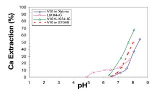
Figure 9—pH dependence of 0.5 M V10 in Xylene, 0.5 M LIX®84-IC in Xylene, 0.5 M V10 and 0.5 M LIX®84-IC in xylene and 0.5 V10 in Shellsol 2046 for Ca at  $40^{\circ}$ C with O:A = 1:1
