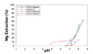
Figure 8—pH dependence of 0.5 M V10 in xylene, 0.5 M LIX®84-IC in xylene, 0.5 M V10 and 0.5 M LIX®84-IC in xylene and 0.5 V10 in Shellsol 2046 for Mg at  $40^{\circ}$ C with O:A = 1:1
