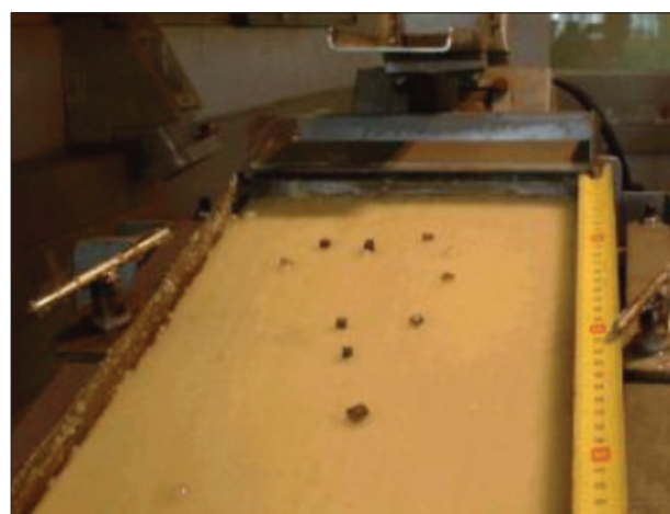
Figure 5—Distribution of diamonds and tracers after agitation
