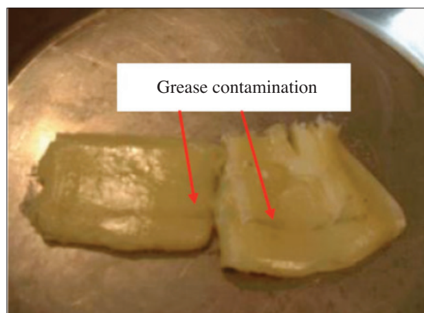
Figure 6—Contaminated grease from river water on the left and the slimes dam water on the right
