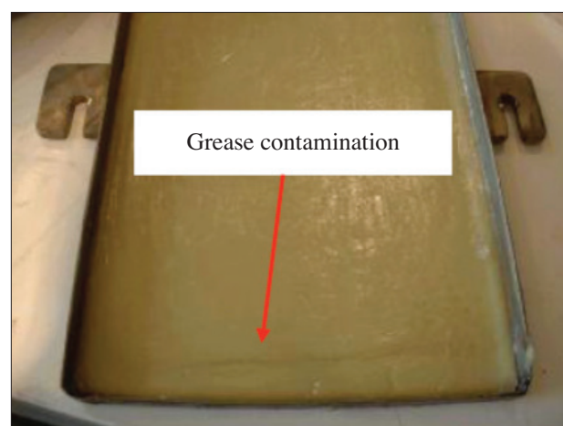
Figure 7—Contaminated grease the filtered dam water
