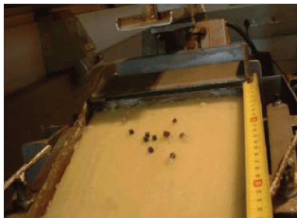
Figure 4—Distribution of diamonds and tracers before agitation
