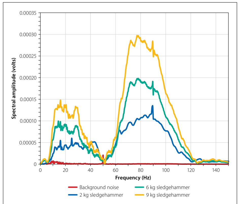
Figure 5 Spectral amplitudes using the Rayleigh wave impact source at 8 m geophone offset
