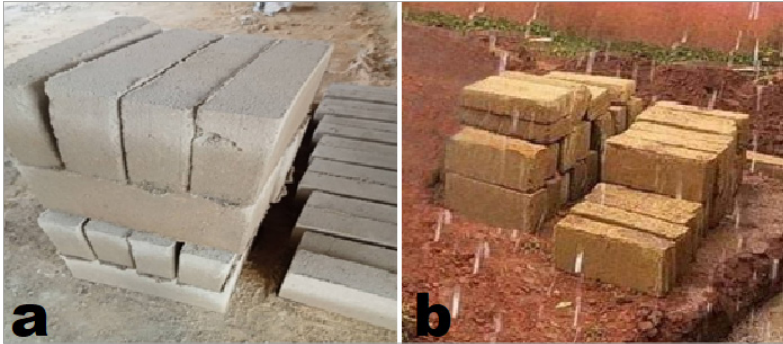
Figure 2a: Stabilised sandcrete blocks
