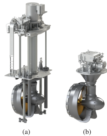
Fig. 7: Azimuth propulsion, (a) L-drive, and (b) Z-drive [21].
