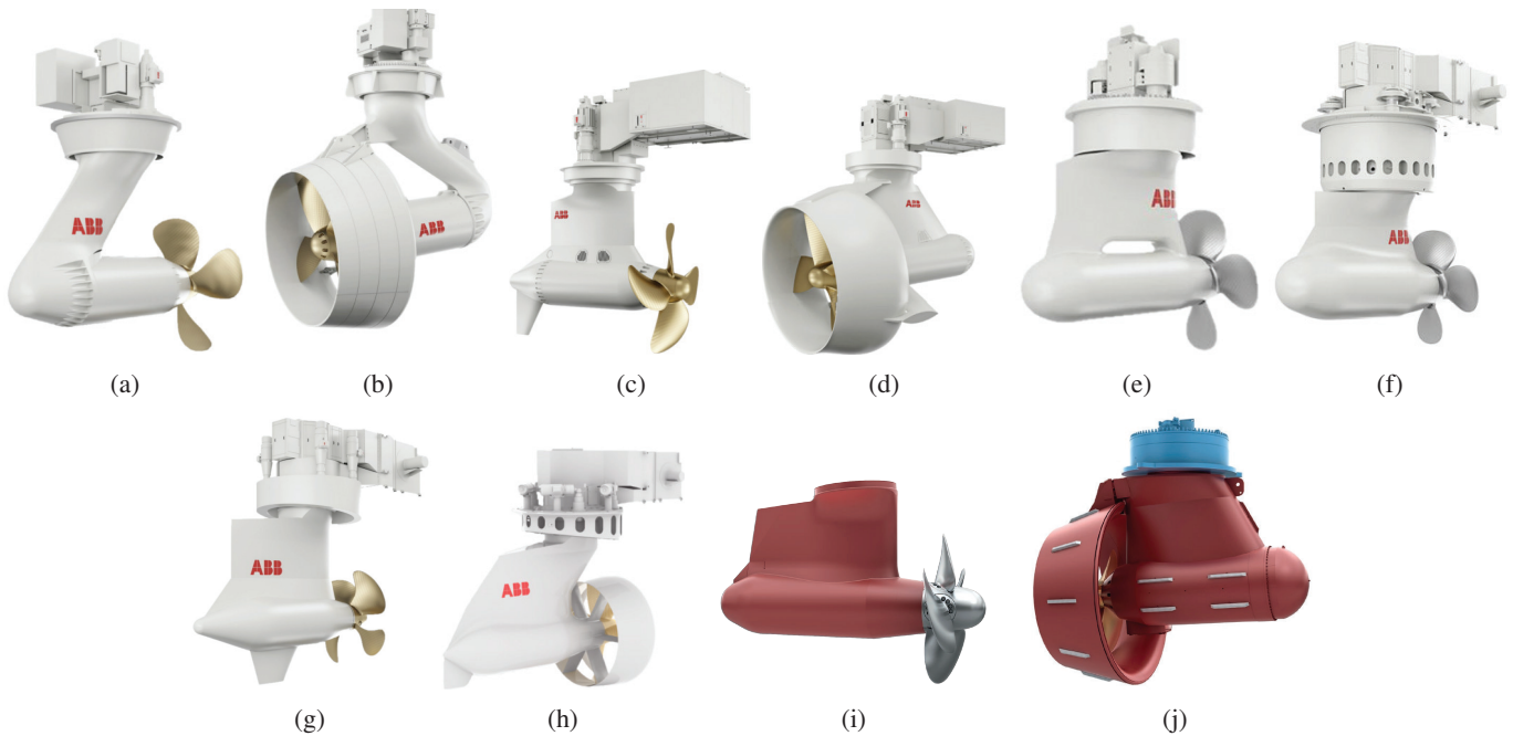
Fig. 8: POD propulsion, (a) Azipod-CO, (b) Azipod-CZ, (c) Azipod-DO, (d) Azipod-DZ, (e) Azipod-ICE, (f) Azipod-VI, (g) Azipod-XO, (h) Azipod-XL, (i) Mermaid ICE, (j) Mermaid PUSH [11], [27].
