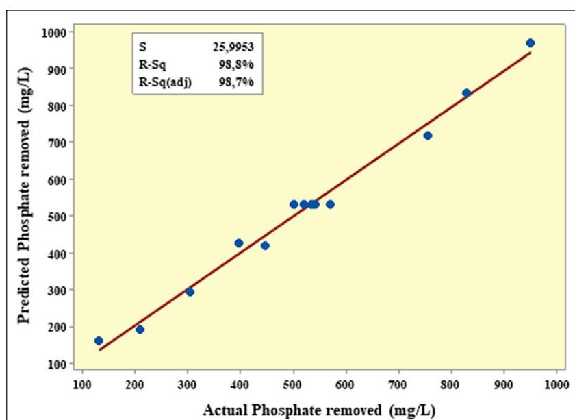
**Figure 6.** Predicted values based on the model in Eq. 1 versus actual values for phosphate concentration
