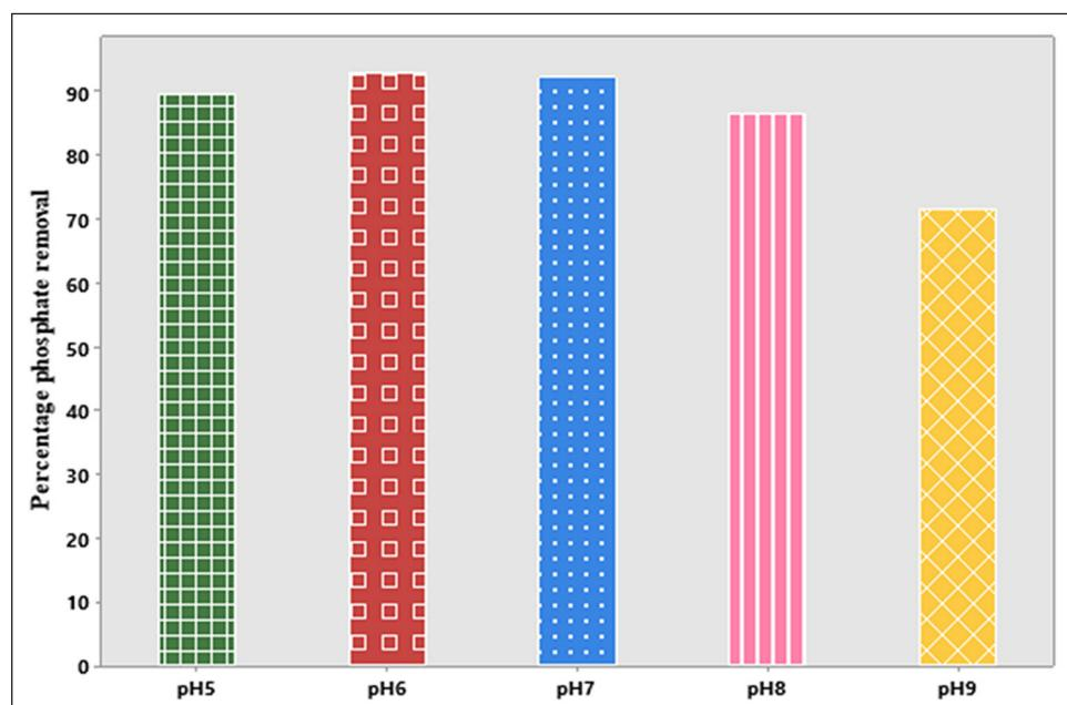
**Figure 3.** Percentage phosphate (PO<sub>4</sub>-P) removal after first 25 minutes of electrocoagulation
