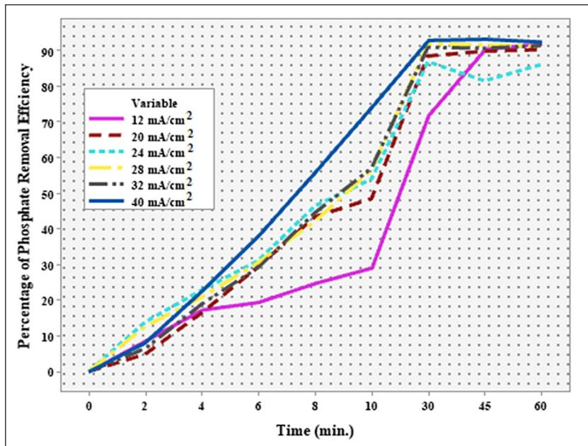
**Figure 1.** Percentage phosphate ( $\text{PO}_4\text{-P}$ ) removal versus time for different current densities
