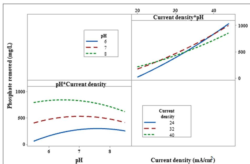
**Figure 5.** The effect of parameter interactions on phosphate concentrations
