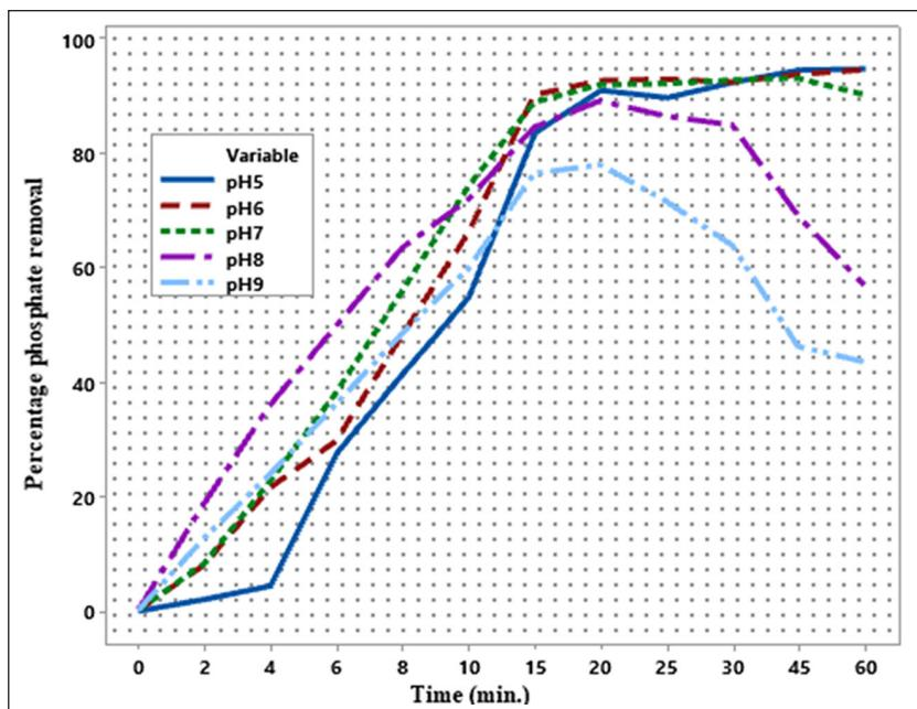
**Figure 2.** Percentage phosphate ( $\text{PO}_4\text{-P}$ ) removal versus time at different initial pH values
