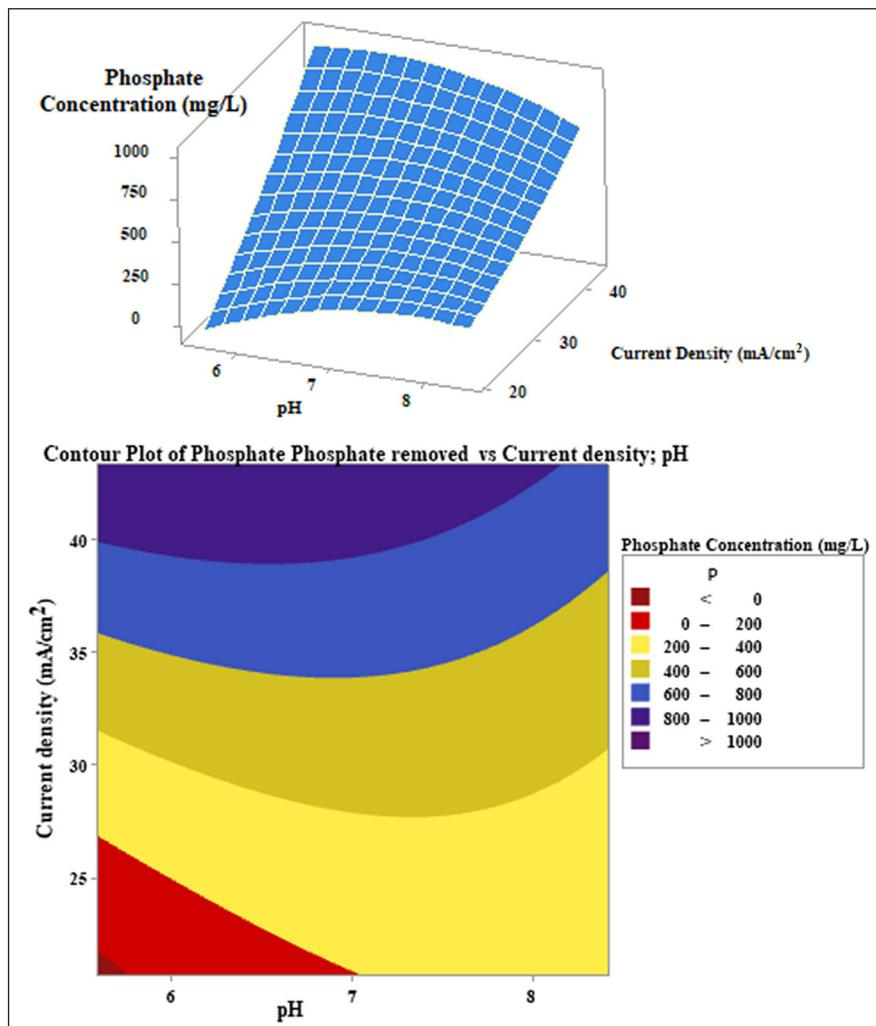
**Figure 7.** 3D Surface and contour plot of phosphate concentration vs current density and pH
