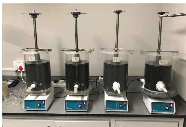
Figure 2. Augmented biosulphide potential (AugBSP) test equipment
