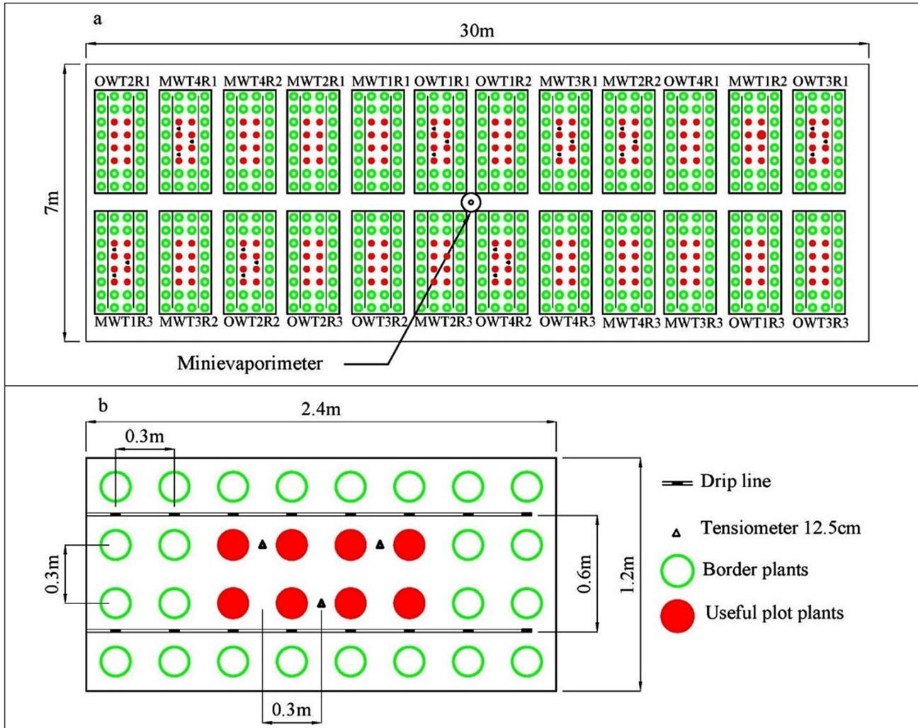
**Figure 1.** (a) Treatment distribution in the experimental area and location of tensiometers. (b) Details of the equipment distribution in the beds, and designation of the useful plot (8 plants) and the border plants
