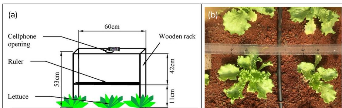
**Figure 2.** (a) Scheme of the structure used to take photographs of the plants in the experiment., (b) Example of a photo taken with details of the graduated ruler and the plants (b).
