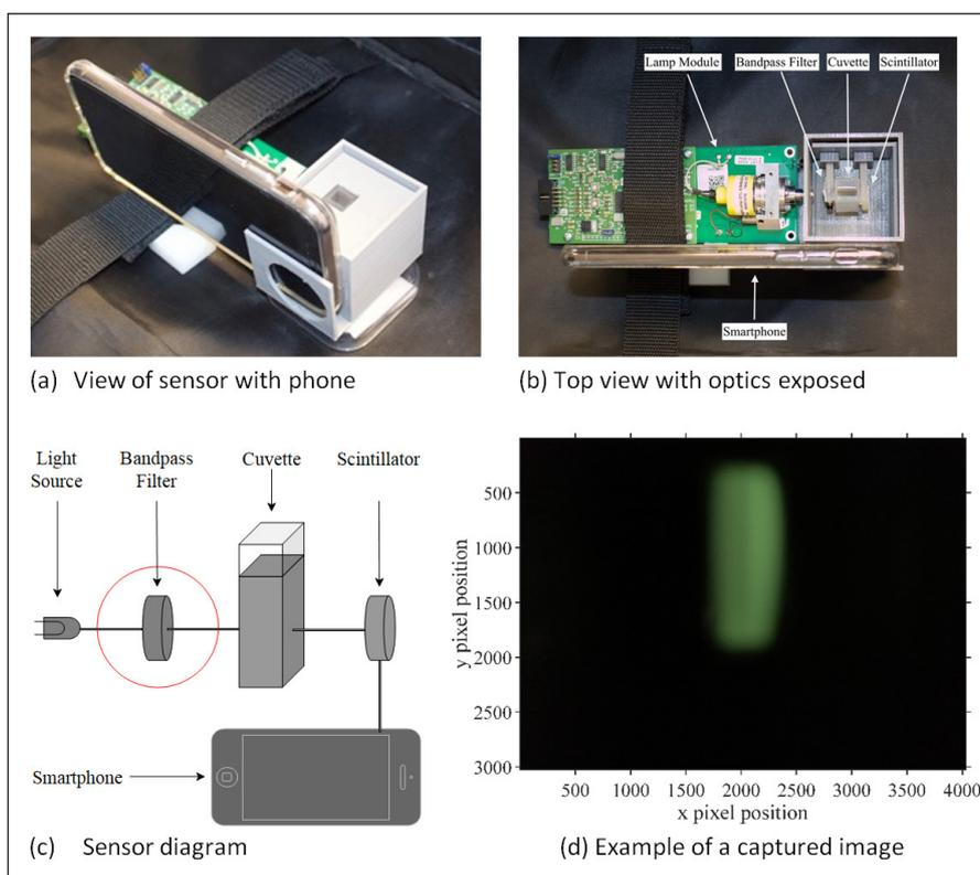
**Figure 1.** Diagram and prototype of smartphone-based nitrate sensor with captured image. The basic components are a deuterium light source, a quartz cuvette, a scintillator and a smartphone camera. The system was evaluated with and without a bandpass filter
