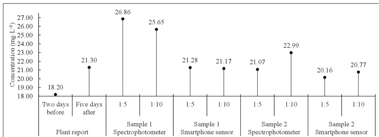
**Figure 3.** Concentrations derived from the diluted effluent water samples, as measured using the AE-560 spectrophotometer and the smartphone-based sensor. Also shown are concentrations of the before and after samples from the wastewater treatment plant report
