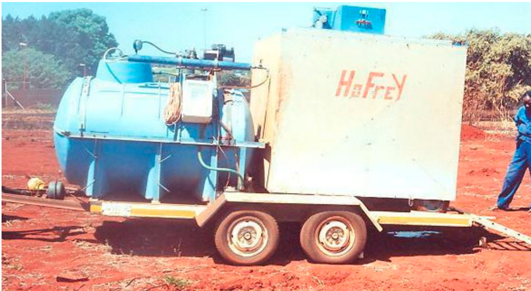
Figure 3.1 (left) Hofrey simulator assembly mounted on trailer
