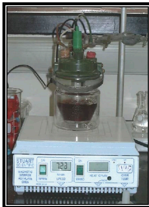
Figure 2 Actual experimental setup for the electro-oxidation reactions
