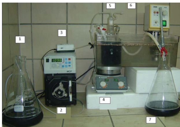
Figure 1 Representation of the experimental set-up used for textile wastewater treatment. 1 - Influent, 2 - Peristaltique pump, 3 - Air pump, 4 - Magnetic stirrer, 5 - Bio réactor, 6 - Bain marie, 7 - Effluent.
