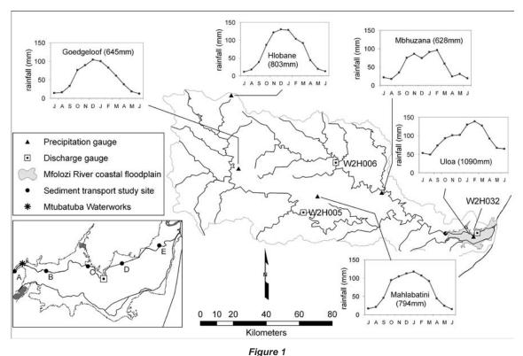
The catchment of the Mfolozi River, showing the location of weather stations, their average monthly precipitation (mm), and average annual precipitation (number in brackets). The location of discharge gauges is also shown. The coastal floodplain study area is displayed on the inset, with the location of the Mtubatuba Waterworks and sediment sampling sites indicated.
