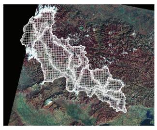
Figure 3 Multiscale grid of the MODCOU spatially distributed flow model applied in the Mesta/Nestos River catchment
