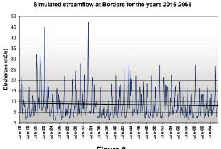
Figure 8 Decrement of simulated runoff based on precipitation data of A2 climate change scenario for the years 2016-2065
