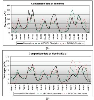
**Figure 6** Comparison between flow rate simulation and data (a) at Temenos, (b) at Momina Kula
