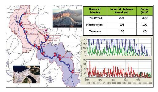
Figure 7 Representation of the Mesta/Nestos River with HEC-ResSim and simulation of the operation of Thyssavros Dam from 1970-1994
