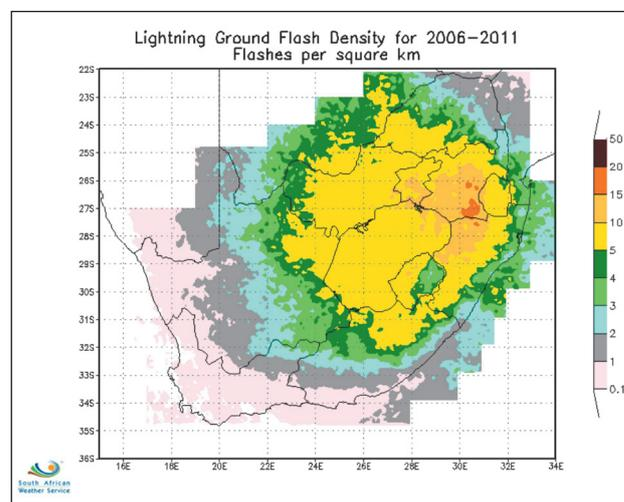
Fig. 1. Lightning ground flash density in South Africa.
