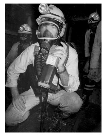
**Figure 7:** SC-100 portable transceiver used by a Rescue Training Station brigadesman wearing a full facemask.
