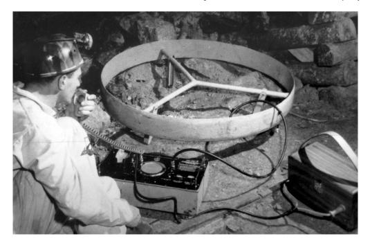
Figure 3: The fresh-air base radio equipment, its battery and multi-turn loop antenna.
