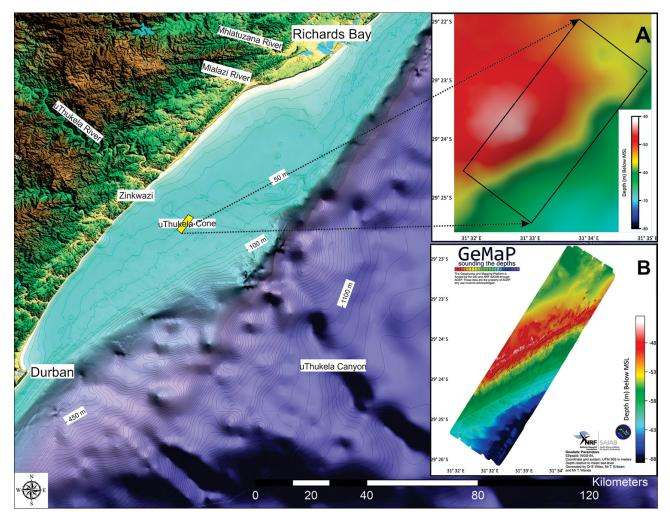
Figure 2: Hydroacoustic surveys of a target area within the uThukela Banks Marine Protected Area. Inset A: Previously available low-resolution bathymetry data<sup>37</sup> (modified). Inset B: Higher-resolved seabed bathymetry from the on-going ACEP Smart Zones Project, offshore Zinkwazi.
