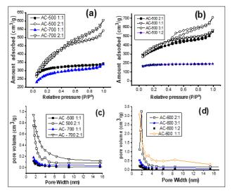
Figure 4: (a) and (b) Adsorption-desorption isotherms of  $N_2$ ; (c) and (d) show the corresponding pore size distribution curve obtained by the Barrett–Joyner–Halenda (BJH) method for AC-500 2:1, AC-500 1:1, AC-700 2:1, AC-700 1:1, AC-600 3:1, AC-600 2:1 and AC-600 1:1.
