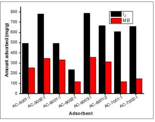
Figure 6: Experimental results for methylene blue (MB) and iodine (I<sub>2</sub>) adsorption.
