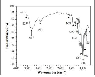
Figure 6: Fourier transform infrared spectrum of SiPCL showing the vibrational modes of bonds related to SiO, and PCL.
