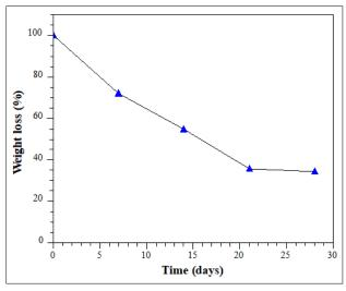
Figure 8: In vitro degradation (weight loss) of SiPCL/TCH soaked in phosphate-buffered saline for 28 days.
