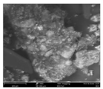
Figure 2: Scanning electron micrograph showing the microstructure of the SiPCL composite.
