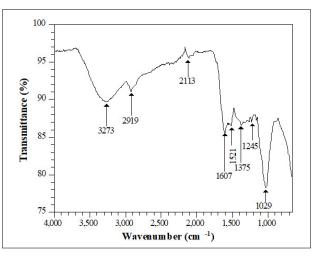
Figure 7: Fourier transform infrared spectrum of SiPCL/TCH confirming the presence of TCH in the SiPCL composite matrix.
