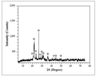
Figure 5: X-ray diffraction pattern of SiPCL/TCH composite showing the presence of TCH in the composite: cristobalite ( $\Phi$ ), PCL ( $\Theta$ ) and TCH ( $\Psi$ ).
