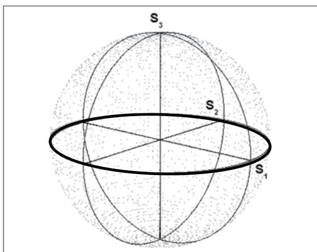
**Figure 5:** This figure shows the compensation of all four states used in the quantum key distribution protocol using one polarisation controller. The S1 axis represents the rectilinear basis, the S2 axis represents the diagonal basis and the S3 axis represents the circular basis. The bold line in the figure, indicated on the equator of the Poincaré sphere, shows that only linear states of polarisation were measured, thus eliminating any ellipticity induced in the fibre channel.
