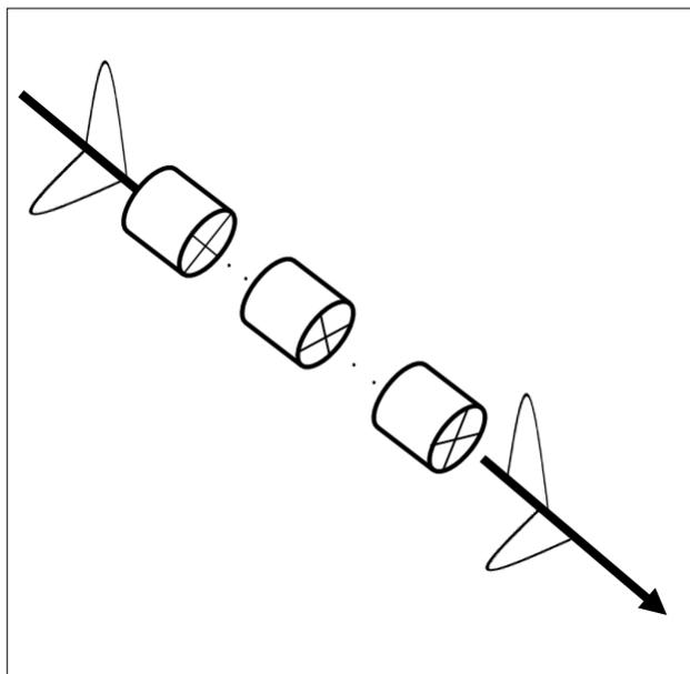
**Figure 2:** Diagram depicting how a state of polarisation is rotated as it is transmitted through a fibre optic cable. The cross sections of the fibre show that the orthogonal components of the state of polarisation are rotated during transmission as a result of their differing speeds. For illustrative purposes, this figure demonstrates a linear rotation, but practically, the fibre can introduce an elliptical element into the state of polarisation as well.
