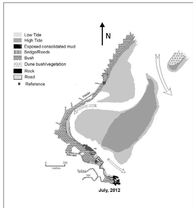
**Figure 12:** Keurbooms Estuary sediment structures after the breach of the new mouth in the northeast. Ebb current flows are indicated.
