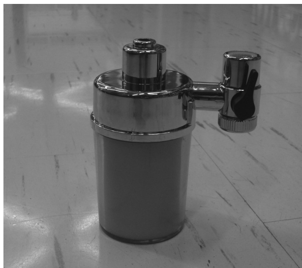
Figure 2: Mini tap filter – a point-of-use water-treatment device – which was used to collect biofilms.
