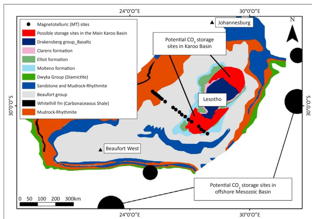
**FIGURE 1:** Map showing the distribution of potential onshore and offshore CO<sub>2</sub> storage sites and the locations of magnetotelluric stations in the Karoo Basin.
