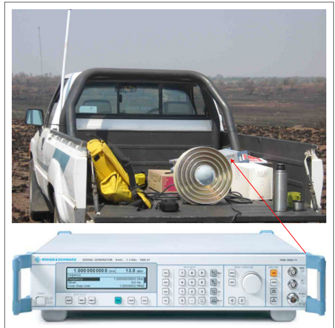
FIGURE 1: The jammer set-up used. A passive choke ring GPS receiver antenna was used as the transmitting antenna and matched the impedance of 50 \Omega of the signal generator on both L1 and L2 frequencies.
